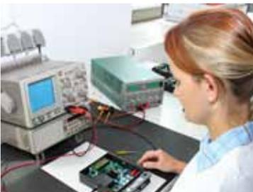
Connection of displays and first quality check of impulse output frequencies
